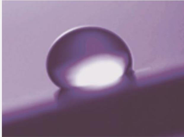
A10 is a patent pending coating with superior hydrophobic properties, which can be applied to most surfaces and materials. A10 can be used for many applications, but is developed to facilitate water droplets rolling off the coated device.
