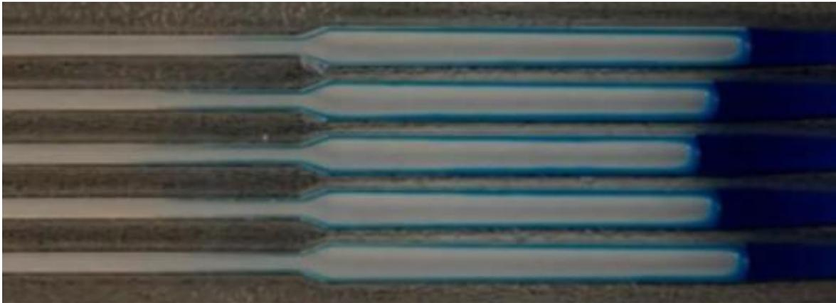
Figure 1. Five parallel channels filled from the right by a blue test liquid (TL1). The pre-shooters at the channel corners are easily seen. For geometrical reasons the channel corners are effectively wetting.
