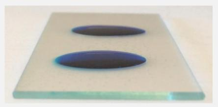
S100 is a patent pending coating with superior hydrophilic properties, which can be applied to most surfaces and materials. S100 can be used for a number of applications, but is developed for single use diagnostic consumables based on capillary microfluidics.
